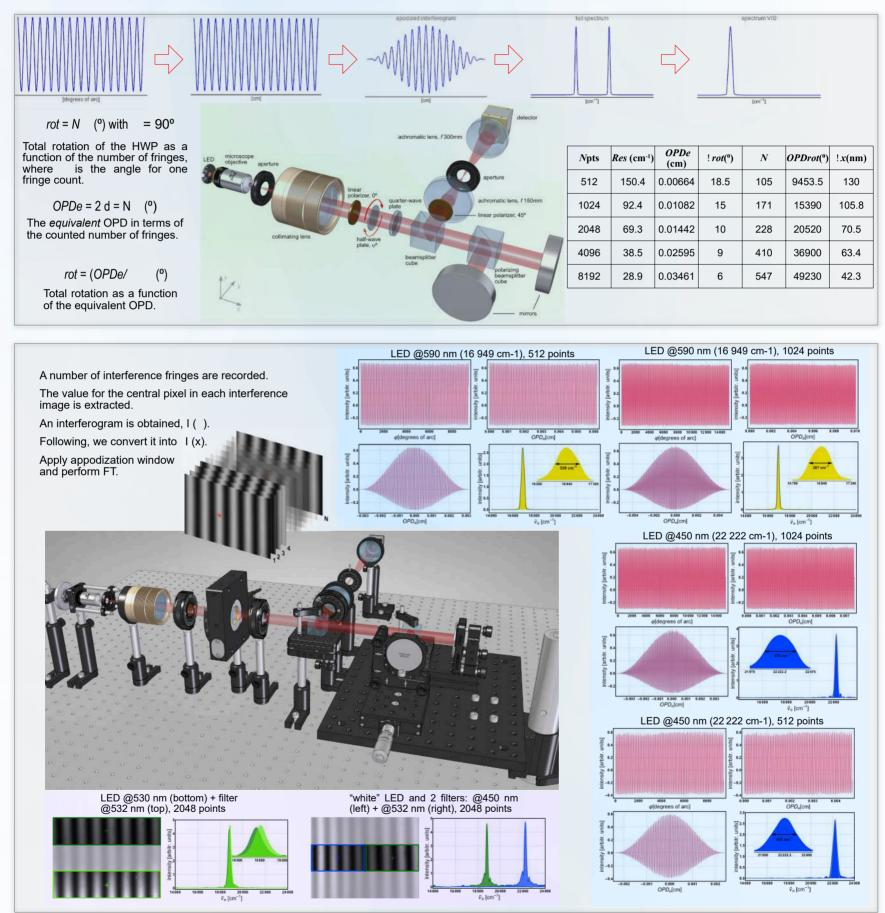
· Geometric phase can be used as a phase shifter mechanism for light measurement using Fourier-transform spectroscopy.
